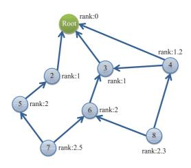
**Figure 8:** In RPL, the network topology (a DODAG) is anchored at the network root. Nodes are placed in the topology according to their rank, which reflects a logical distance to the root. In storing mode, all traffic is routed first upwards until reaching a common ancestor, and then downwards to the destination. For instance, node #2 can send to node #8 through the path: #2, Root, #3, #6, #8.
