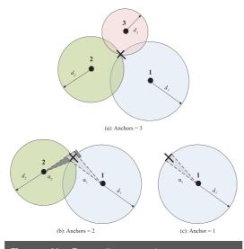
**Figure 11:** Depending on the measurement capabilities of the WSN nodes, the minimal anchor count can be reduced from *three* to *one*. *d* and  $\alpha$ , respectively, represent distance and angle measurements.
