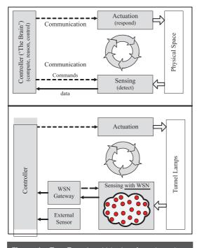
**Figure 1.** Top: Functional blocks of a cyber-physical system (CPS). Bottom: A wireless sensor network (WSN)-based CPS architecture for adaptive tunnel lighting.<sup>1</sup> While the functional description for different components of a CPS design is specific to the application requirement, its architectural abstraction remains the same.
