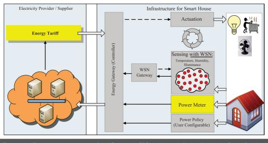
Figure 12: Functional components of a WSN-based CPS architecture for application in Smart Building/ House.
