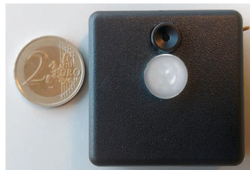
Figure 1: LOCI is of size 5 \times 5 \times 2 \text{ cm}^3 housing thermopile and PIR sensors.
